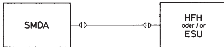
Fig. 3-4 Test setup for harmonics measurement
