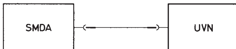
Fig. 3-8 Measurement of modulation-generator output voltage
