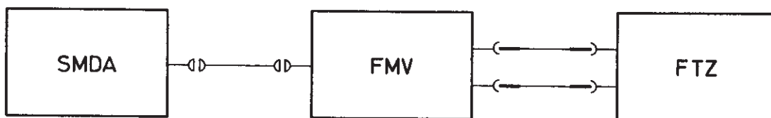
Fig. 3-16 Measurement of modulation distortion with FM and \phi M
